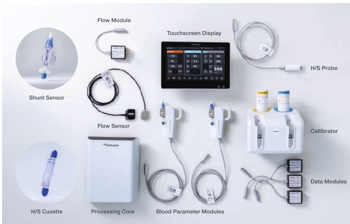
Figure 2: Components of the CDI OneView Monitoring System.
